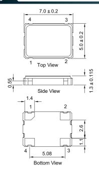
PAD FUNCTION: 1: ENABLE CONTROL 2: GND
